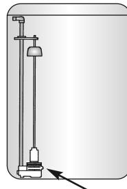
The 464 shut-off prevents air from entering the Simplus system during the draw cycle. It also maintains the proper water level in the chlorine regeneration tank.
